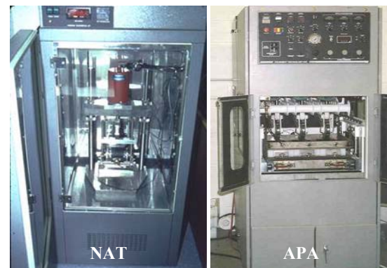
FIGURE 28 Nottingham Asphalt Tester (NAT) Used to Determine Resilient Modulus ( M_r ) and Asphalt Pavement Analyzer (APA) Used to Determine Rutting Resistance, Fatigue Endurance, and Moisture Damage.
